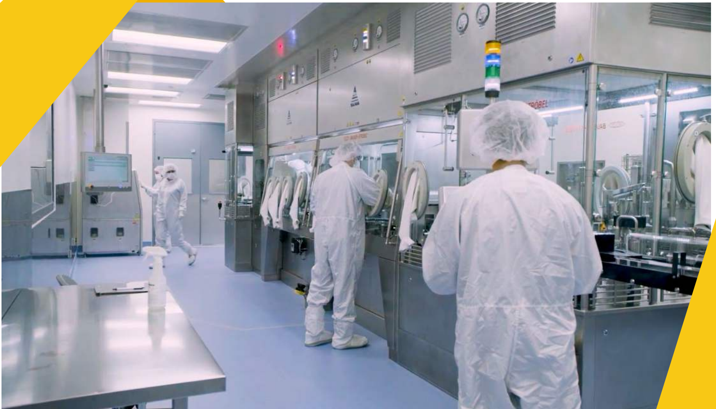
Argonaut’s fully isolator-based filling line (shown above) separates operators from the aseptic process, delivering higher sterility assurance and significantly reducing particulate risk, reject rates, and potential batch loss.
